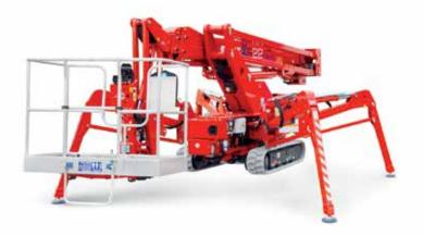
Articulated platform with a pantograph and a telescopic boom with two extensions plus Jib. A combination that, thanks to the articulated stabilizers, makes the S22HD the undisputed queen of work in extreme conditions. A unique platform.
